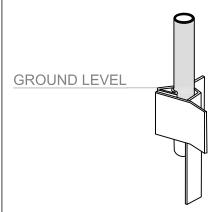
FOR EARTH OR ASPHALT **INSTALLATION** USE V-LOK VR-2 (MODEL 23 ROUND) OR APPROVED **EQUAL**
