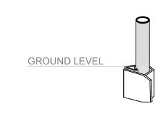
FOR CONCRETE INSTALLATION USE V-LOK VR-1 (MODEL 23 ROUND) OR APPROVED EQUAL
