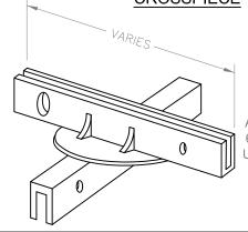
FOR STREET NAME SIGNS WITH 4-INCH LETTERING, USE SUPR-LOK 990-X OR APPROVED EQUAL. FOR 6 INCH LETTERING, USE **ULTRA SUPR-LOK 12CRX** OR APPROVED EQUAL.
