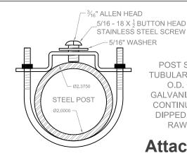
POST SHALL BE TUBULAR 2.375-INCH O.D. GLOSS **GALVANIZED STEEL CONTINUOUS MILL** DIPPED, WITH NO RAW ENDS.
