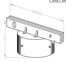
FOR STREET NAME SIGNS WITH 4-INCH LETTERING, USE SUPR-LOK 922-X OR APPROVED EQUAL. FOR 6 INCH LETTERING, USE **ULTRA SUPR-LOK 1238X** OR APPROVED EQUAL.
